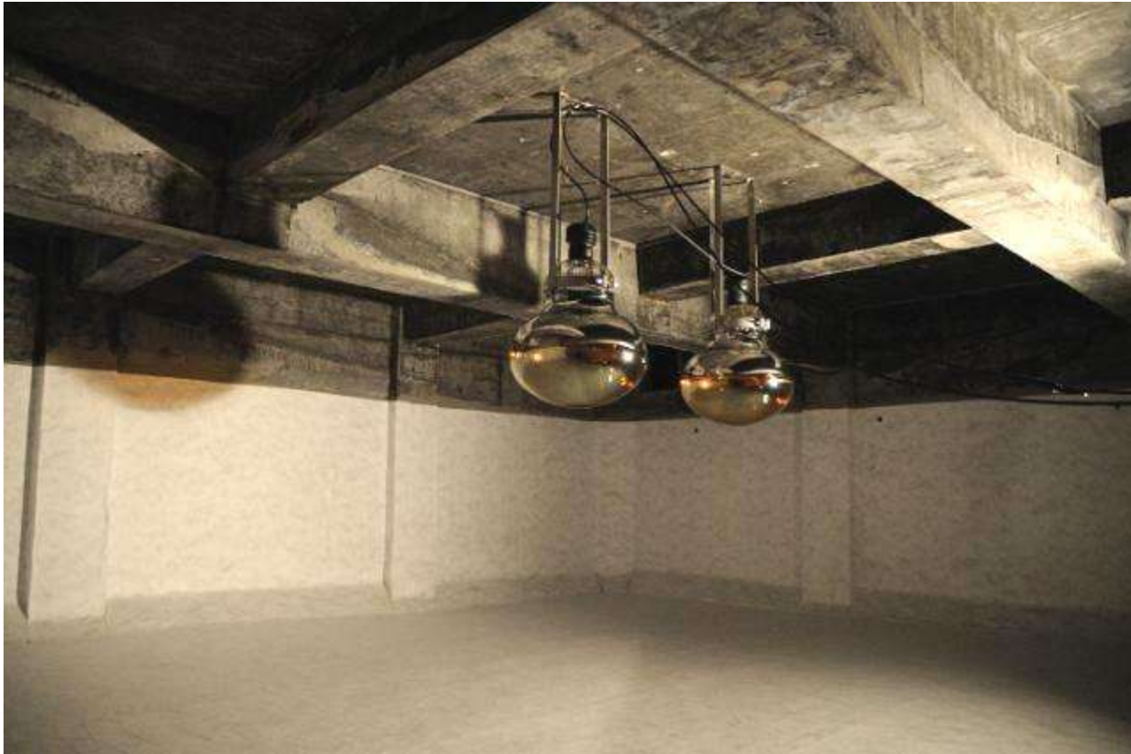
Tyvek sheet walls and two 20 inch PMTs
